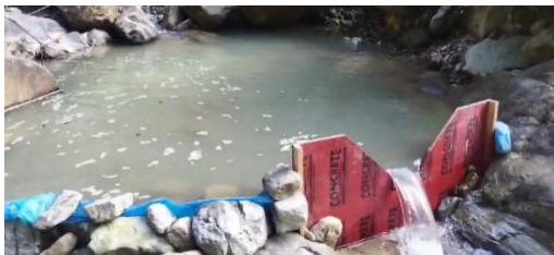
Use of V-notch to measure discharge
